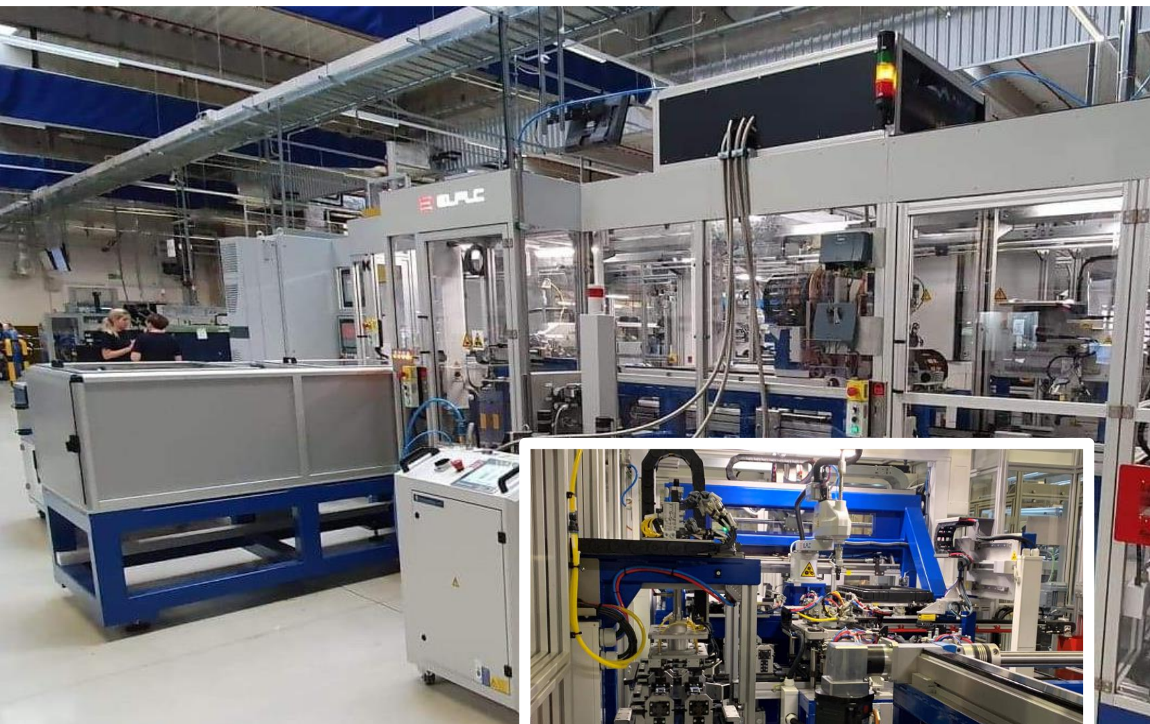
Heating elements (emobility) production line (Poland)
